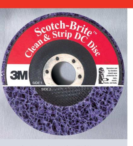
Scotch-Brite™ Clean and Strip XT DC Discs are constructed from a tough non-woven nylon web impregnated with silicon carbide mineral and bonded together with a phenolic resin. On one side of the disc is a fibreglass depressed centre plate for attachment to angle grinders.
